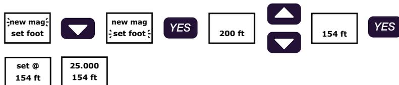
Note: a magazine needs to be installed, locked in its running position, for you to have access to the magazine footage setting.
