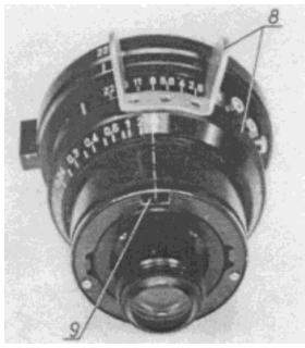
III. Turn tens focusing ring(Fig. 5/8) to Infinity mark, so that the middle of the retaining pin slot (Fig. 5/9) is opposite the stop.
