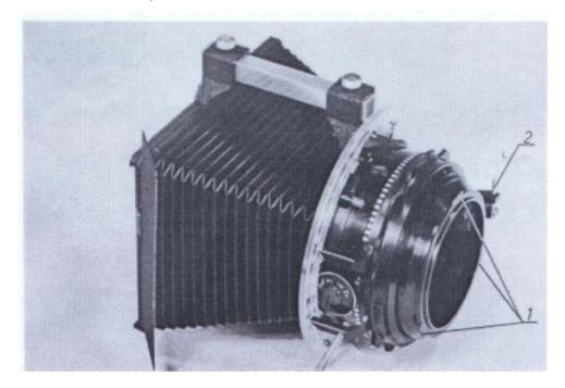
1. Universal Lens Blimp, Fig, 2, with the three clamping lugs (Fig. 2/1) in the three grooves on the camera (as for zoom lenses)I then turn to right until the lens blimp engages the latch (Fig. 2/2) The matte box is mounted exactly as on zoom lenses.
